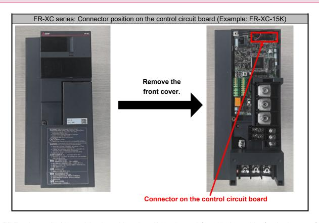
(2) For the applicable models, the cable color will be changed from black to white for the harness for connection between the main circuit board and the control circuit board.
